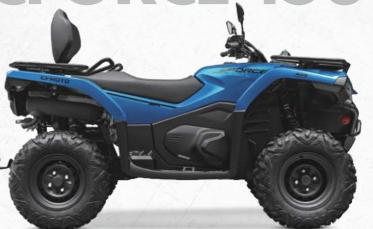
CFMOTO answers the call of customers looking for an affordable, rugged and maneuverable midsize machine that's built tough with the CFORCE 450. Its quality starts with a high-strength steel-frame backbone, matched to a proven single-cylinder liquid-cooled SOHC engine and smooth CVT transmission.
